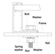
Figure 6. Bolt installation methods
