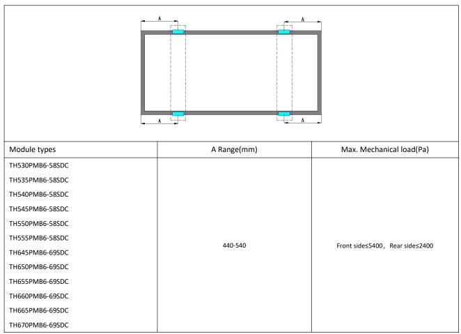
Eight clamps mounting on long side of frame and rails perpendicularly to the long side frame
