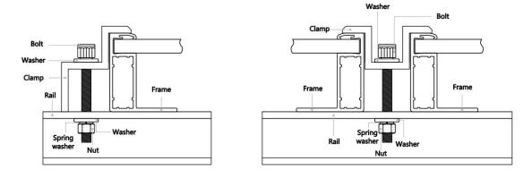
Figure 7. Specific installation of clamps
