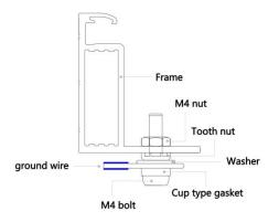
Figure 1. Ground hole and its identification
